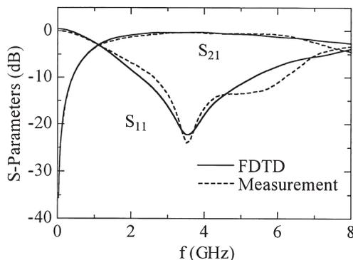
**Fig. 6** Simulated and measured S-parameters of the microstrip line interconnect using bonding ribbon and dielectric pad with  $\epsilon_2 = 10.2$ ,  $t = 0.6$  mm and  $l = 4$  mm. Other parameters are the same as in Fig. 2.
