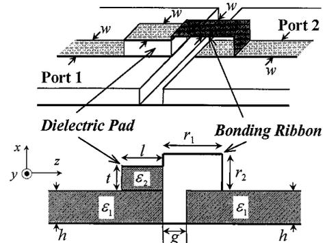
**Fig. 1** Microstrip line interconnect through a gap using a bonding ribbon and dielectric pad.
