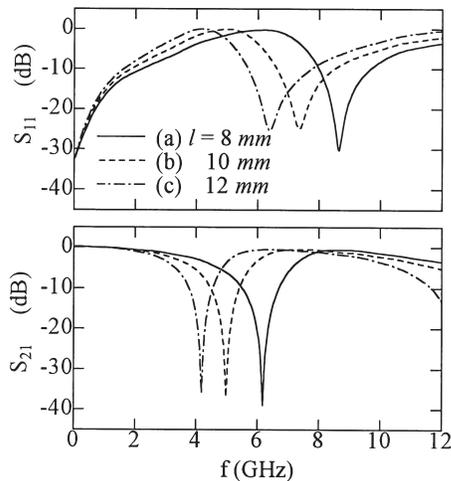
**Fig. 10** S-parameters obtained by FDTD simulation for the DC pass microstrip line interconnect where the length of the dielectric pad is a parameter. Other parameters are the same as in Fig. 9. (a)  $l = 8$  mm, (b)  $l = 10$  mm, (c)  $l = 12$  mm.
