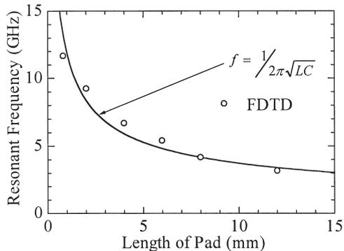
**Fig. 5** Resonant frequencies of the interconnect with respect to different lengths of dielectric pad. Other parameters are the same as in Fig. 3.
