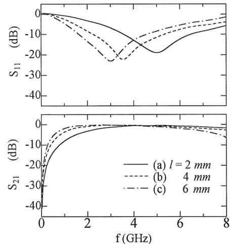
**Fig. 7** S-parameters obtained by FDTD simulation for the microstrip line interconnect using bonding ribbon and dielectric pad with  $\epsilon_2 = 10.2$  and  $t = 0.6$  mm where length of the pad as a parameters. Other parameters are the same as in Fig. 6. (a)  $l = 2$  mm, (b)  $l = 4$  mm, (c)  $l = 6$  mm.
