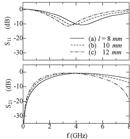
**Fig. 4** S-parameters obtained by FDTD simulation for the microstrip line interconnect using bonding ribbon and dielectric pad with  $\epsilon_2 = 2.33$  and  $t = 0.8$  mm where length of the pad as a parameters. Other parameters are the same as in Fig. 3. (a)  $l = 8$  mm, (b)  $l = 10$  mm, (c)  $l = 12$  mm.
