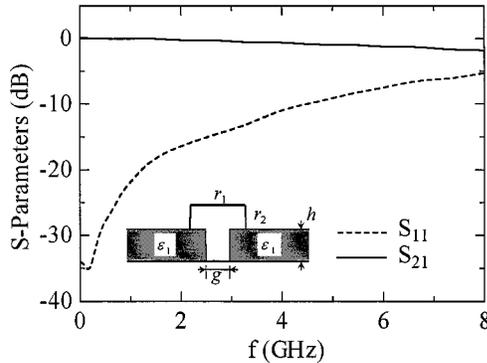
**Fig. 2** Coupling characteristics of two microstrip lines connected by conventional ribbon bonding. ( $g = 1.6$  mm,  $h = 0.8$  mm,  $\epsilon_1 = 2.33$ ,  $r_1 = 4$  mm,  $r_2 = 1.4$  mm and  $w = 2.3$  mm).
