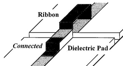
**Fig. 8** Microstrip line interconnect with top conductor of dielectric pad and microstrip are connected.
