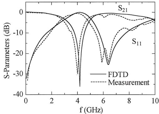
**Fig. 9** FDTD simulation and measurement results of S-parameters for the modified microstrip line interconnect. The parameters are the same as in Fig. 3.
