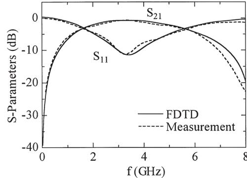
**Fig. 3** FDTD simulation and measurement results of S-parameters for the microstrip line interconnect using bonding ribbon and dielectric pad with  $\epsilon_2 = 2.33$ ,  $t = 0.8$  mm and  $l = 12$  mm. Other parameters are the same as in Fig. 2.
